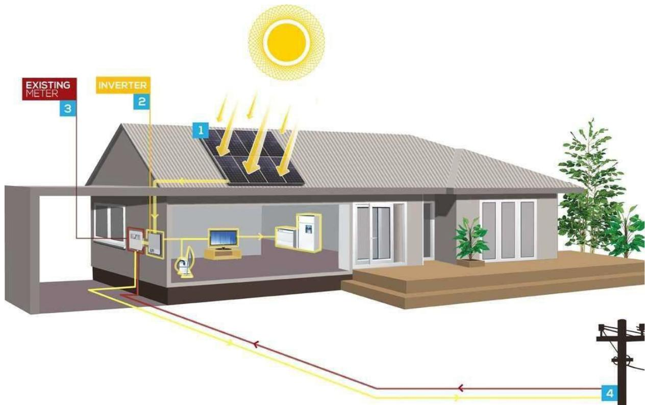
Solar PV panels, usually fitted to the roof, convert sunlight into direct current (DC) electricity. The number of panels installed will depend on the nominal size of your system. Collectively groups of these panels are referred to as a solar array.
